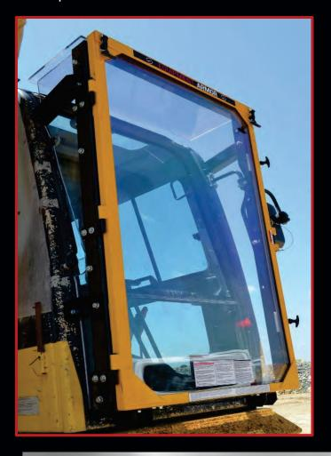
"Because the Equipment Armor shield frame sits at 90 degrees to open and close like a door, the windshield was exposed to greater potential damage. The subframe wrap eliminated windshield breakage. One of our customers estimated the sub-frame wrap alone saved him from \$1,200 to \$1,800 a year in broken windshields, not to mention down time..."
