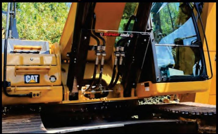
In response to our customer's requests, Equipment Armor, Inc. developed a Hydraulic Cylinder Guarding System designed to protect both hydraulic hoses and fittings from fly rock. In addition to preventing machine damage, the Hydraulic Cylinder Guard also aids in protecting operators from flying hydraulic hoses cut loose under pressure and the unsafe situations that can be created by leaking hydraulic lines.
