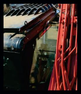
Equipment Armor responded to the injury of a hydraulic hammer operator in Tennessee by developing a line of custom boom side glass overlays and replacements.
